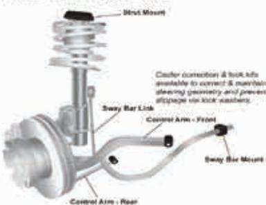
Caster correction & lock kits available to correct & maintain steering geometry and prevent allpage vehicle systems.
